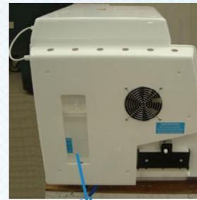
Pressure Relief Tank
