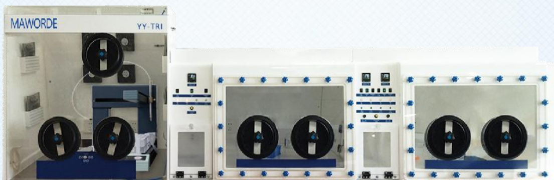
Customised Anaerobic Workstation (L: Protein purifier, R: Integrate with shaker and ELISA)
