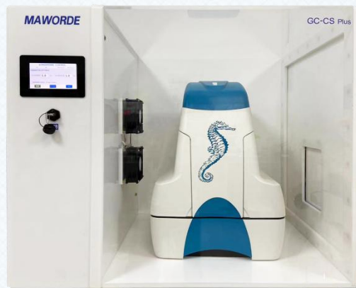
Integration of Seahorse into a Hypoxia Incubator
