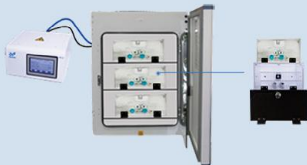
Chambers can be controlled by a single controller and each chamber can be set to different O 2 or CO 2 concentration
